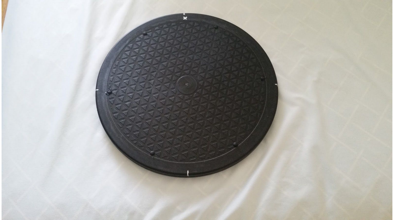
Figure 5: Our Lazy Susan with appropriate markings for rotation ( 0^\circ , 90^\circ , 180^\circ , 270^\circ )
