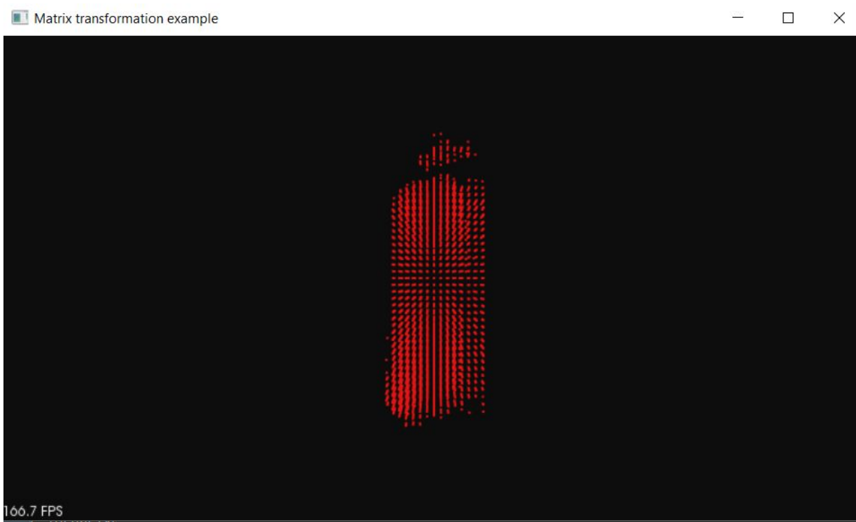
Figure 6: Horizontal view of point cloud achieved by registering snapshots of point clouds from the left side of the water bottle.
